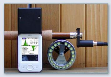
The entire *Fly Casting Analyzer System*: a sensor capsule, a small cable that connects the capsule to the (black) circuit box, the circuit box, and an attached Palm Pilot. A casting signature can be immediately analyzed using the Fly Casting Analyzer software installed on the Palm.
