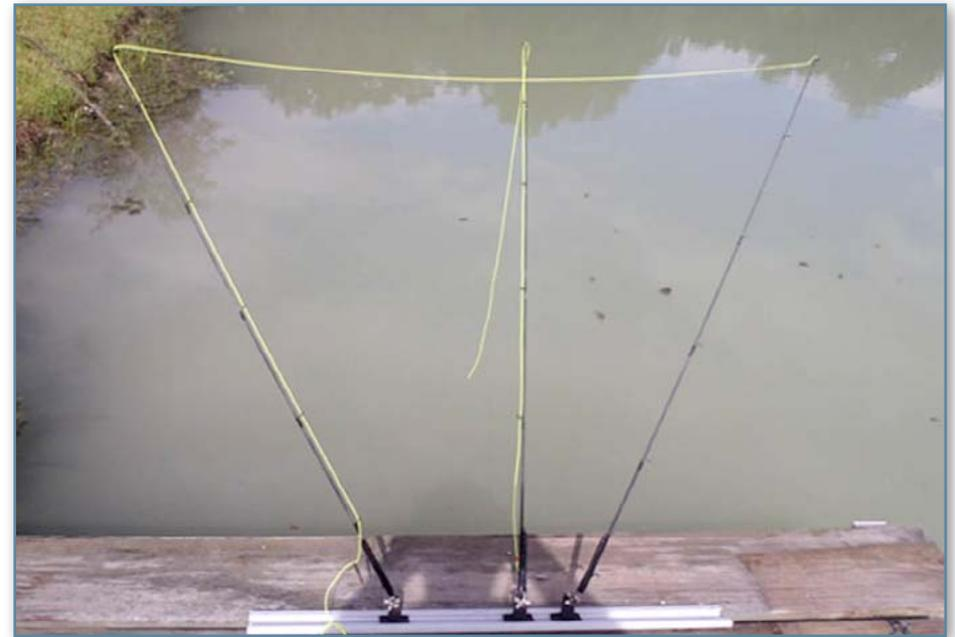
tips on either end represent the rod stop positions of the cast. By adjusting the wing nuts at the base of the rods and tilting their position, you are able to adjust them to either open up or decrease the casting arc of the cast. Likewise, by moving the rods closer together or spreading them apart, you are able to illustrate adjustments to the casting stroke. By tilting the base (sliding bar) of the device you are able to illustrate changes in trajectory and/or
